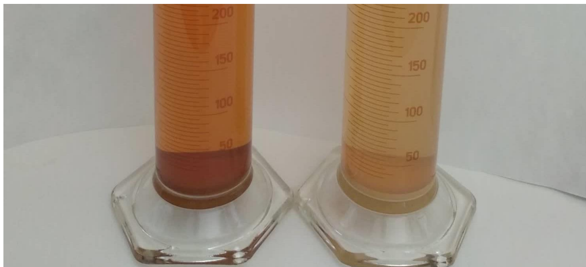
Fig. 11. Sediment volume after bacterial oxidation of \text{Fe}^{2+} , precipitation and sedimentation of \text{Fe}(\text{OH})_3 on the left and jarosite on the right. Concentration of dissolved \text{Fe}^{3+} in the liquid phase: 2357 \text{mg L}^{-1} , sample on the left and 1516 \text{mg L}^{-1} , sample on the right
