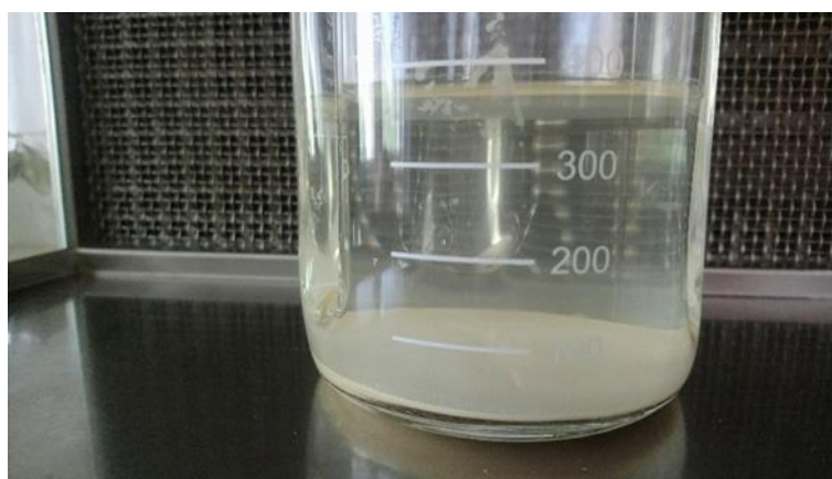
Fig. 11. Sediment after bacterial oxidation of \text{Fe}^{2+} in mine water from Nižná Slaná and precipitation of K-jarosite. \text{Fe}^{2+} concentration at the beginning 5087 \text{mg L}^{-1} . After complete oxidation of \text{Fe}^{2+} to \text{Fe}^{3+} , the concentration of dissolved \text{Fe}^{3+} in the liquid phase was 208 \text{mg L}^{-1} , pH 1.9
